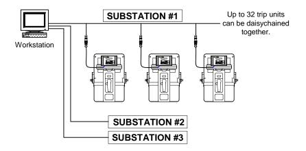
As system demands grow, additional twisted pairs of wire can be added, each twisted pair capable of supporting an additional 32 AC-PRO or ZERO-Hertz communicating trip units. The host PC can also be connected to a Local Area Network (LAN), allowing other computer sites access to AC-PRO information.
